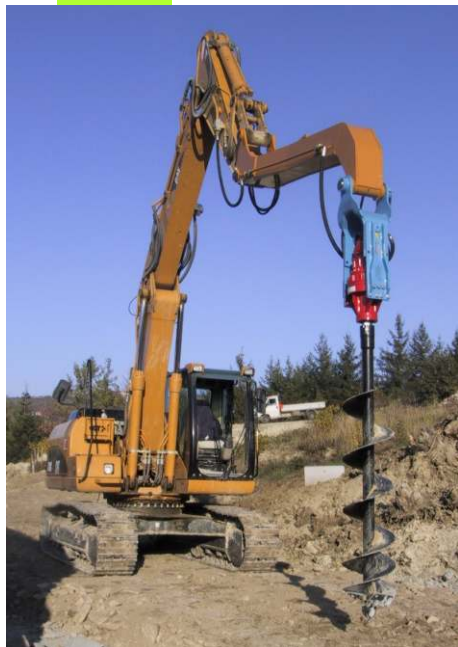
Trivelle per i Escavatori fino a 30 ton. Hydraulic drill for excavators up to 30 tons.
